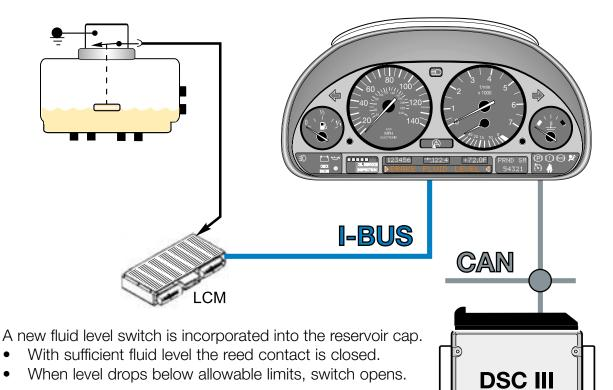
Since the normal position is closed, this circuit is monitored for shorts to + and ground.
